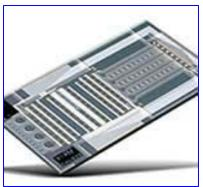
A researcher mixes a DNA sample with a polymerase enzyme and DNA primers and passes it through a bank of 12 microscopic channels, each measuring 150 -200 microns, within the silicon. Electrical heating elements that are embedded resistors in the silicon, heat the
