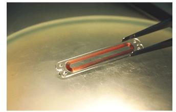
CardioMEMS, a member of Georgia Tech's Advanced Technology Development Center (ATDC), is pioneering a BioMEMS sensor to monitor heart patients. They have combined wireless technology with BioMEMS to provide doctors with more information while making testing less
