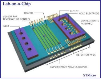
Lab-on-a-chip allows small amounts of bodily fluids to be tested in seconds. All chemical
