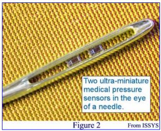
sensors that are designed for medical applications. ISSYS is developing intelligent BioMEMS sensors and systems to enhance the quality of medical treatment that can apply to:
