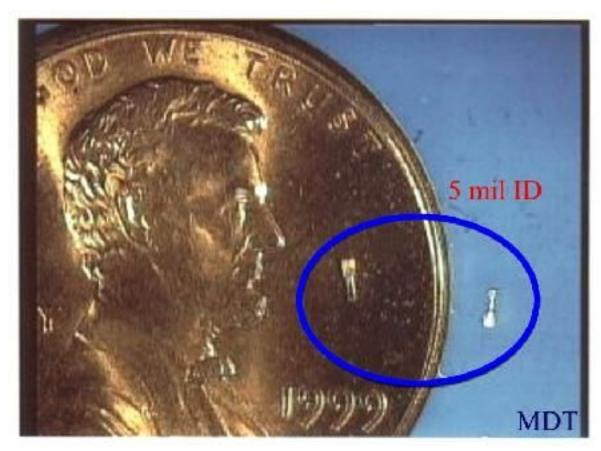
Figure 4 - Tiny Micro-molded Part
