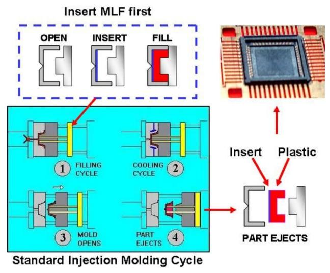
Figure 5 - Insert Molding Process
