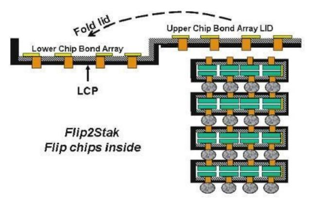
Figure 15 – Flip2Stak Design
