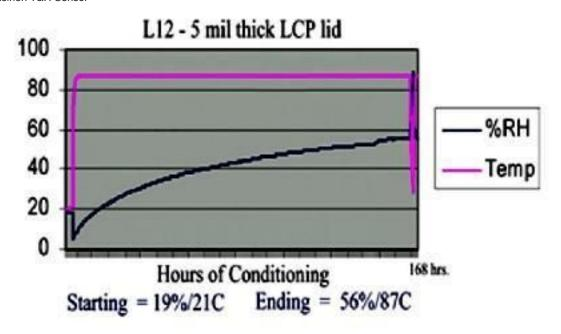
Figure 12 – T&H Curve for Sealed Packages at 85%rh/85oC
