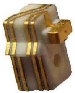
Figure 17 - 3D Molded Antenna
