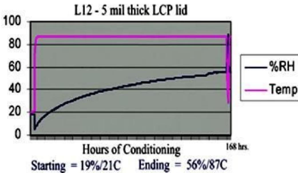
Figure 12 – T&H Curve for Sealed Packages at 85%rh/85oC
