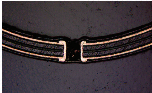
Example of a “gradual” bend in a flex circuit.
